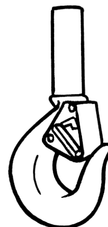
Self-Closing Flapper Latch (Shank Hook)
