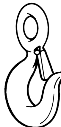
Self-Closing Flipper Latch (Eye Hook)
