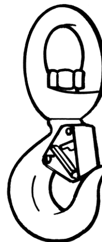
Self-Closing Flapper Latch (Swivel Hook)
